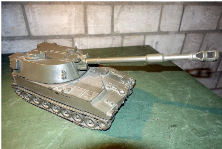
Pz Hb 79/95 KAWEST (Modell) – 1979/1998-heute; 23.7 to (leer); V8 2-Takt Dieselmotor 405 PS; 15.5 cm Haubitze (max. 28 Km); 1 Mg 7.5 mm; 6 Mann – Bestand: 348 Stk.
